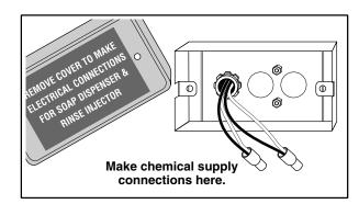
Figure 21: Chemical Supply Connection
