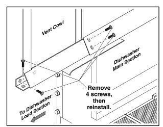
Figure 4: Load Belt Roller Guard Extension
