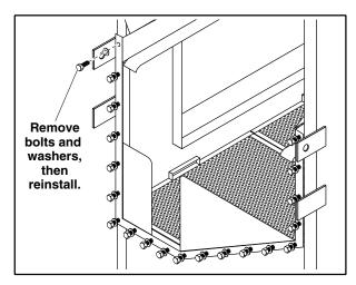
Figure 2: Load End Tank Mount
