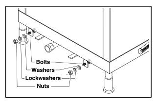
Figure 7: Unload End Frame Mount
