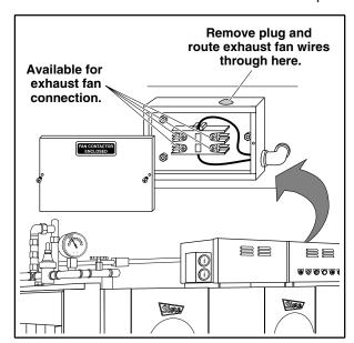
Figure 18: Exhaust Fan Electrical Connection
