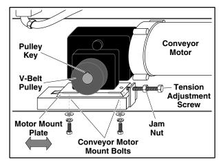
Figure 9: Conveyor Motor V-Belt Tension Adjustment
