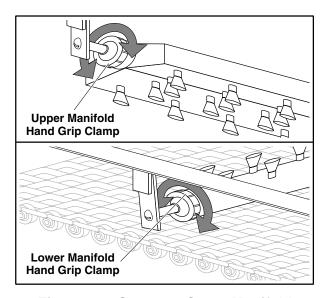
Figure 27: Scrapper Spray Manifold Hand Grip Clamp
