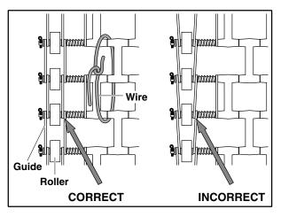
Figure 13: Conveyor Peg Belt Assembly
