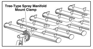
Figure 28: Tree-Type Spray Manifold Mounting Clamp Handle
