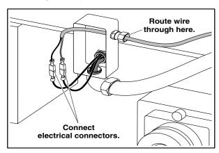
Figure 15: Conveyor Stop Bar Switch Electrical Connection
