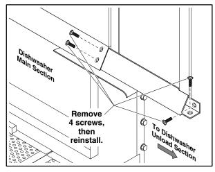
Figure 8: Unload Belt Roller Guard Extension
