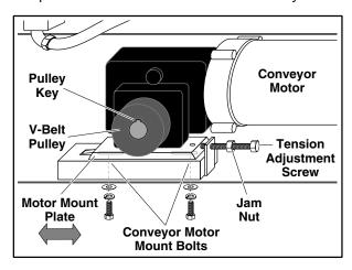
Figure 22: Conveyor Motor V-Belt Tension Adjustment
