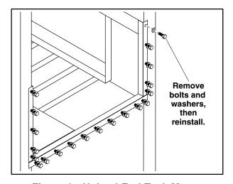
Figure 6: Unload End Tank Mount
