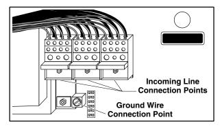
Figure 20: Main Electrical Connection
