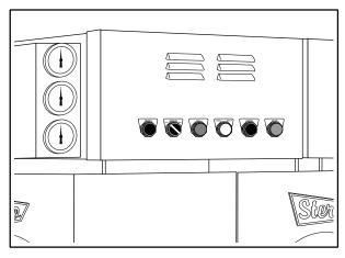
Figure 23: Operating Controls Location
