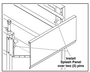
Figure 5: Splash Back Panel Installation
