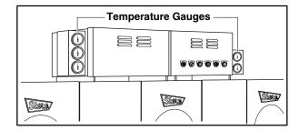
Figure 25: Temperature Gauge location
