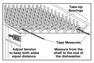
Figure 14: Take-up Bearing Adjustment
