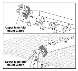
Figure 26: Scrapper Spray Manifold Mount Clamp
