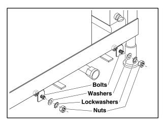
Figure 3: Load End Frame Mount
