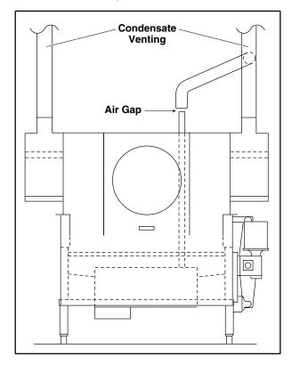
Figure 17: Recommended Gas Venting
