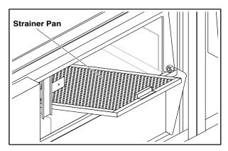
Figure 31: Strainer Pans Removal
