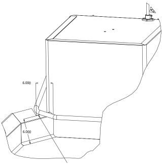
A NOTCH MUST BE ADDED TO BACKSPLASHES OVER 6" HIGH ON CORNER MACHINES TO PREVENT INTERFERENCE WITH DOOR MECHANISM. NOTCH MUST EXTEND 6" FROM FACE OF THE MACHINE.
