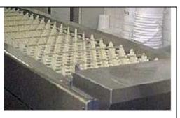
Conveyor Belt to have Cross Rods every 4<sup>th</sup> Row to eliminate racks getting stuck in fingers of conveyor belt.
