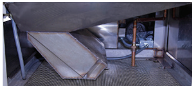
Welded, stainless steel, perforated under carriage prevents access to the bottom of the machine.
